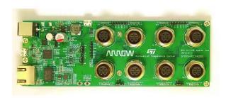
with demo application showing the simplicity to connect to 8 IO-Link devices via STM's L6360 – the IO-Link communication master transceiver IC.
